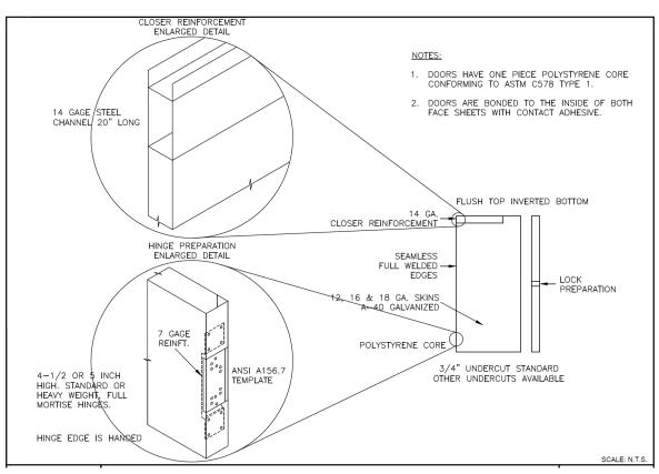
Rocky Mountain Metals Inc, 1703 Hollow Metal Door with Polystyrene Core Bullet Resistant, UL 752 Level 3 9.4.18
