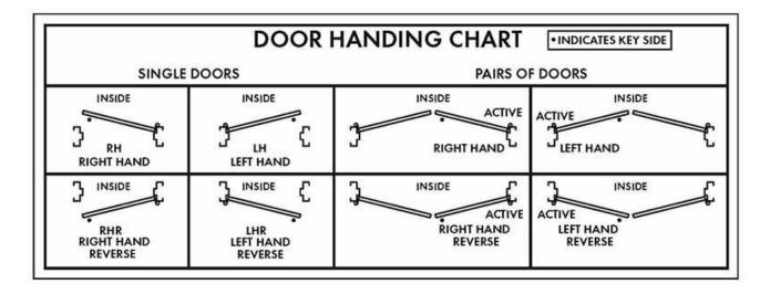
The "handing" of a door refers to the direction that the door swings. It is important to know the correct handing of your opening when ordering Doors, Frames, Exit Devices and other hardware. The hand of the door is determined by the secure side (the side which you initially unlock and enter) of the door.
